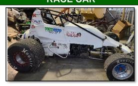
Sprint Car, complete with 360 NON ASCS engine and wing Extra rear tires for spring car
